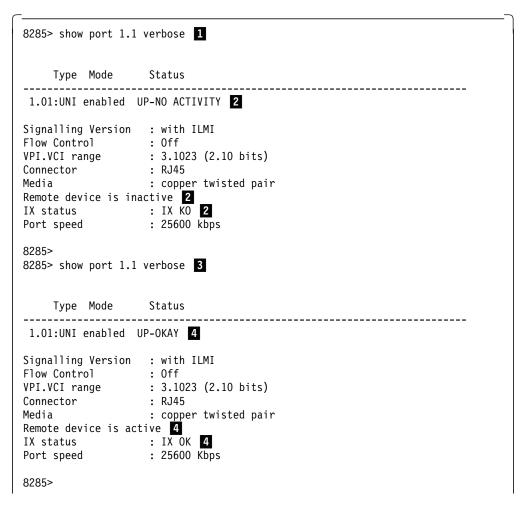
Figure 45. The Sample Console Screen to Check the Physical Connection
